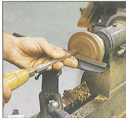
Photo I Shape the inside of the lid. For best results, work the gouge from the center to the outside edge.
