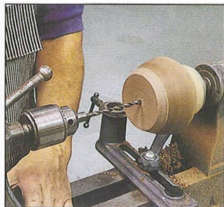
Photo L Mount a drill chuck on the lathe tailstock, and drill a \frac{1}{4} " hole \frac{5}{16} " deep into the lid for the knob's tenon.
