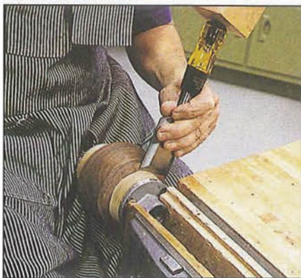
Photo J Holding the faceplate in the bench vise, separate the box from the backing block along the paper joint.
