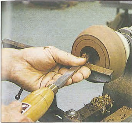
Photo G Turn the inside of the box. Use a rule to check depth, a pair of calipers to check wall thickness.
