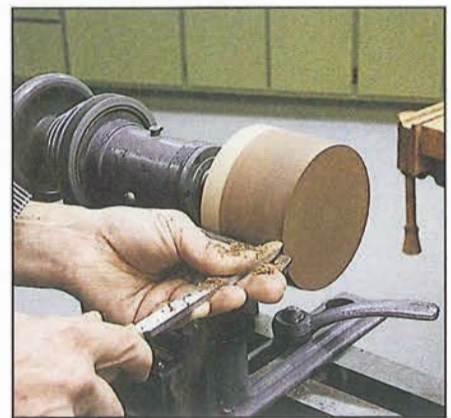
Photo B With a roundnose scraper, round down the blank before you form the box contour.
