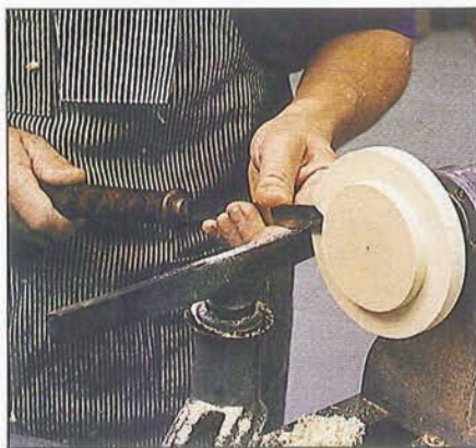
Photo N Using your parting tool, cut a lip into the backing block to accept the box.
