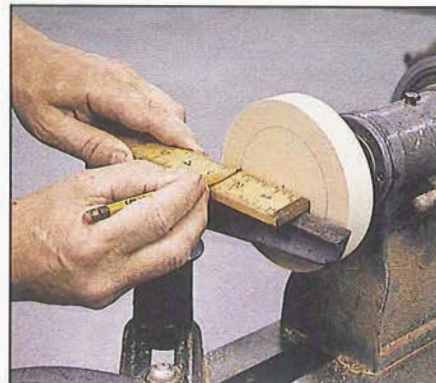
Photo M Mount a fresh backing block, then lay out the centerpoint and the box's inside diameter on it.
