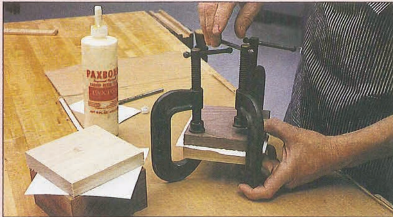
To make a paper joint, glue a sheet of notebook or typing paper between the blank and backing block, and clamp until the glue dries.
