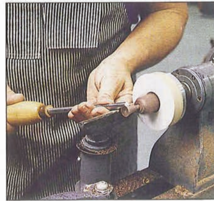
Photo P To form the knob, bore a 1 1/8" hole into the backing block, insert the blank, then turn the knob to shape.
