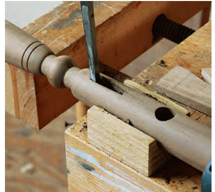
Chop out the crest rail mortises in the back posts with a 1/4" mortising chisel. Make the mortises 9/16" deep and 1 1/2" long. Use a curved support to brace the post from below and to keep it from twisting.
