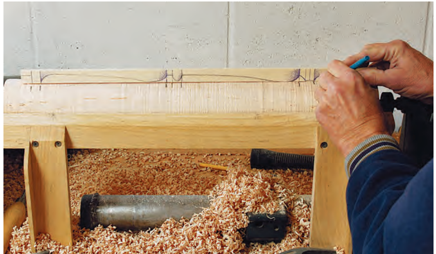
Before beginning any new piece of furniture, the author makes a set of story sticks. This piece required two such sticks. One is a pattern for the cabriole leg profile, and the other is the stick shown above, on which the elements of the turned pedestal have been marked off.
