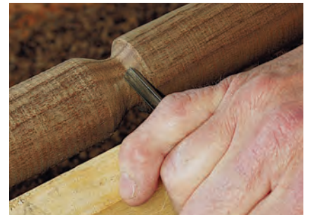
Form the cove at the base of the front-post vase with a 3/8" fingernail gouge. Begin with the gouge standing on its side facing the cove. Then roll it 90 degrees into the cove until it lies on the rest with the flute up.
