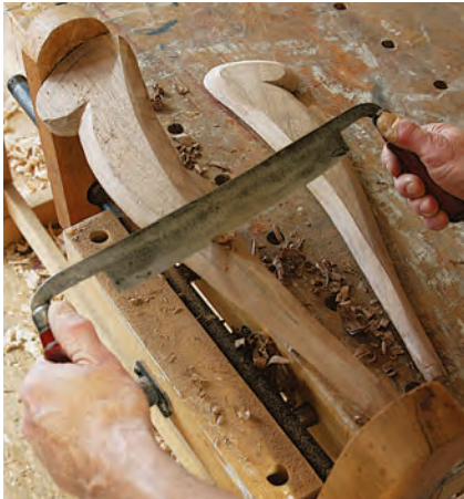
The author turns to a drawknife, rasps and sanding to shape the edges of the arms. Pencil lines establish the transition areas.
