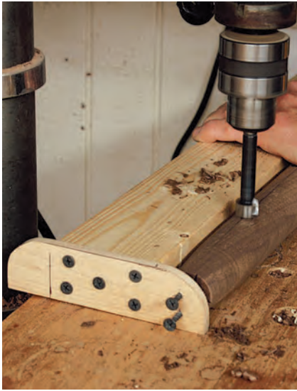
Bore holes for the front and back rung mortises on the drill press with an oversized table supporting the FRMJ. Set up the drilling depth first, testing it on same-diameter scrap.
