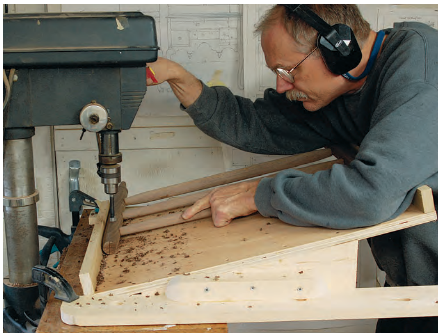
After you've glued your front ladder together, set up the side-rung-mortise jig (SRMJ) as shown so that it will bore a 15/16"-deep mortise in the center of the posts. Then drill the three side-rung mortises in one post, turn the ladder around, and drill the three side-rung mortises in the other post. Next, rotate the jig 180 degrees on your drill press table and drill the side-rung mortises in the back ladder.
