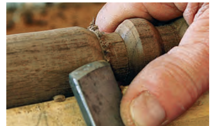
Roll half beads with the bottom half of your skew chisel. Engage the work you're rounding with the skew at a 45° angle, then roll it over the section so that the stroke is completed with the skew standing on-edge on the rest.
