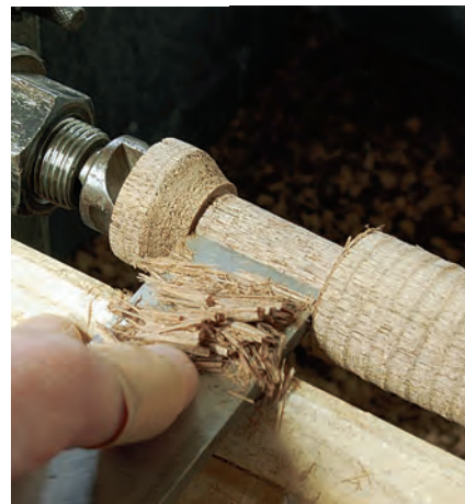
Finish the tenon with a bevel-side-down paring chisel. Aim for consistent tenon thickness and a slightly loose fit. Cut off the end waste.
