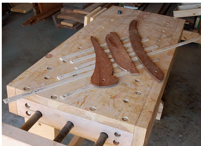
This set of story sticks constitutes the templates our author uses for this rocker. The three cherry parts are traceable patterns for arms, rockers and crest rail. The four sticks near the top are rung sticks on which the tenon lengths are indicated. The other two sticks represent the front and back posts. Those sticks index rung locations, finial and vase shapes and post diameters at various points along their lengths.
