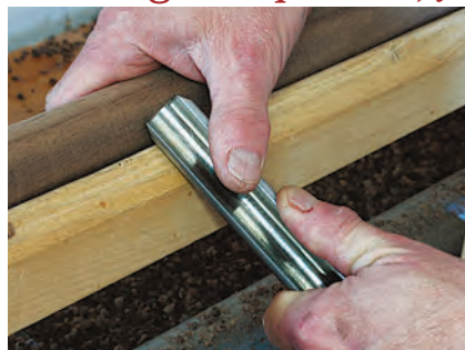
The author uses his free hand to support the back of thin spindles when he turns them to shape. It reduces flexing and excess vibration.
