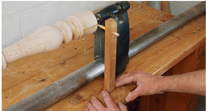
This simple marking gauge allows the author to draw marks on a turned spindle that are perfectly parallel to its axis of rotation. To mark the locations of the leg mortises, he stops the lathe's rotation by engaging the locking pin on its indexing head. He then slides the jig (pencil point pressing lightly against the object) along the bed to scribe a straight line.
