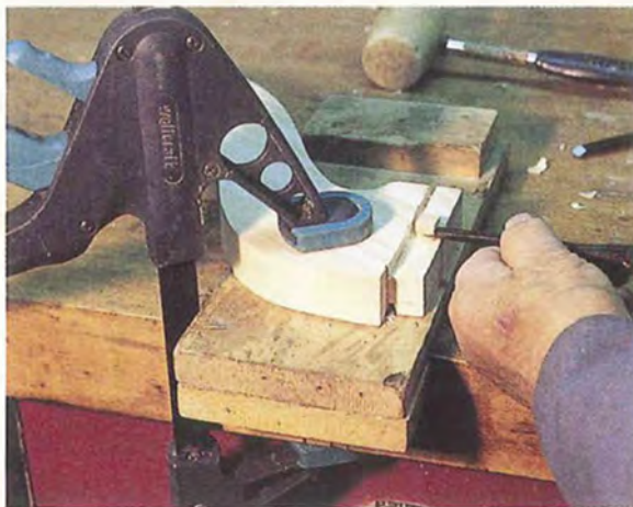
Once the shoulder cuts are made, the author uses a chisel to shape the dovetails to fit the sockets in the pedestal perfectly. Chisel in the direction of the wood grain and use a padded clamp.
