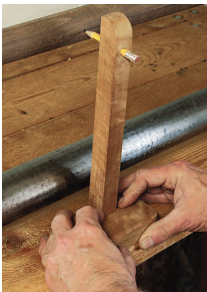
This marking jig allows the author to draw mortise lines along the posts that are parallel to the axis of rotation. He first locks the lathe's indexing head, then slides the jig along the lathe table while keeping the pencil point engaged with the work.
