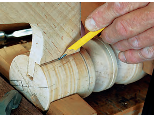
Square tenon shoulders won't mate tightly with a rounded pedestal. To create a tighter fit, the author bevels the areas underneath the shoulders. Here, he's marking these areas.
