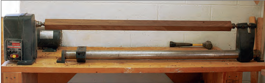
The author's modest Craftsman lathe is modified with a bed extension and wooden length-of-part toolrests. He also added gravel to each of the shop-made columns supporting the lathe.
