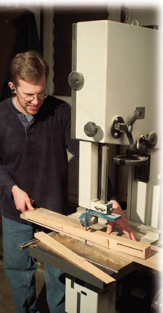
The legs receive tapers on two adjacent faces. Mark these faces to avoid miscuts, and rip the tapers using a commercial or shop-made tapering jig. The author made these cuts easily on the hand saw.
