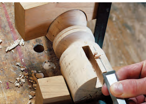
With a wide chisel, create the bevels that will lie under the leg shoulders. These bring the shoulder up tight against the pedestal base. Pare carefully to your layout lines, checking the fit periodically.
