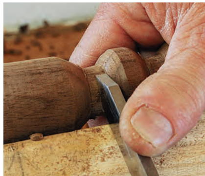
Use a parting tool to create the two filets on either side of the bead at the base of the finial. Steady the post with your hand.
