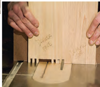
Cut the drawer face pins and slots first (above photo). Then use the drawer face to set the first offset for the drawer side joints (right photos).
