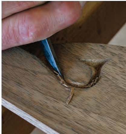
The author details the crest rail with decorative carvings using a sharp knife and paring chisel, followed by careful sanding.
