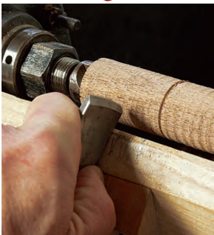
The author transfers the lengths of the rungs from the story sticks directly onto his wooden tool-rests, then to the work with a skew chisel.
