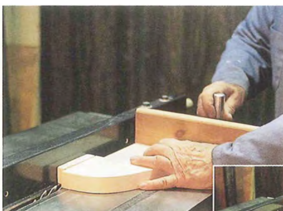
To ensure straight shoulders on the tails, the author created two jigs to hold each leg exactly square as he formed the shoulder of the dovetail. The curve in the leg is matched by the shape of the jig (inset photo) to hold the legs securely as they are being machined.
