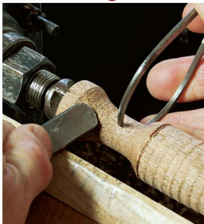
Reduce the tenon nearly to final size with a fingernail-ground spindle gouge, checking its diameter periodically with calipers.
