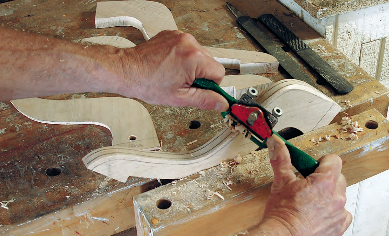
The cabriole legs on the original candlestand have slightly crowned bevels on either side of their top edges. The author created these bevels with a spokeshave and a rasp, as shown above, after first freehanding some guidelines with a pencil.
