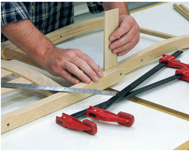
Sizing the leg set to exactly fit between the backrest members is critical. To allow for 1/8" on each side for washers, use a piece of 1/4" scrap as a feeler gauge. Adjust the length of rungs to give the leg set a perfect fit.
