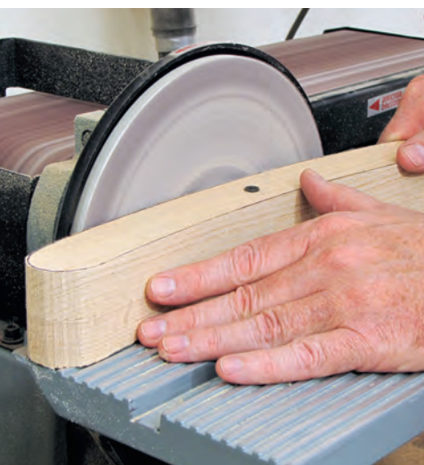
With all components cut out, refine the curves smoothly by sanding down to the marked line. A benchtop disc sander easily handles outside curves, while an oscillating spindle sander takes care of inside curves. Following that, do the finish sanding by hand in combination with a random orbit sander.
