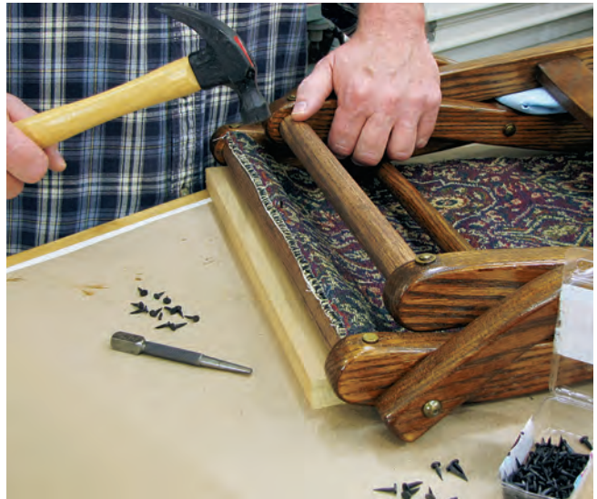
A row of steel tacks secures the seat fabric in place. Note that the author used a piece of scrap to solidly support the seat stretcher while tacking. There are two layers of fabric on this chair to improve its strength.
