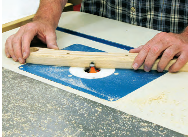
A roundover bit mounted in a router table is used to ease the edges of all the chair's components. All four edges of each leg and armpiece receive the roundover; it helps the chair look, feel (when you sit) and work better.
