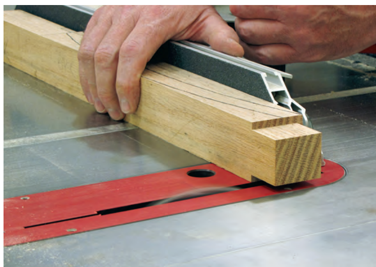
To give you more control and to allow the workpiece to run squarely over your table saw's dado cutter, mill the tenons on the ends of the backrest stretchers before cutting them to the curved shape.
