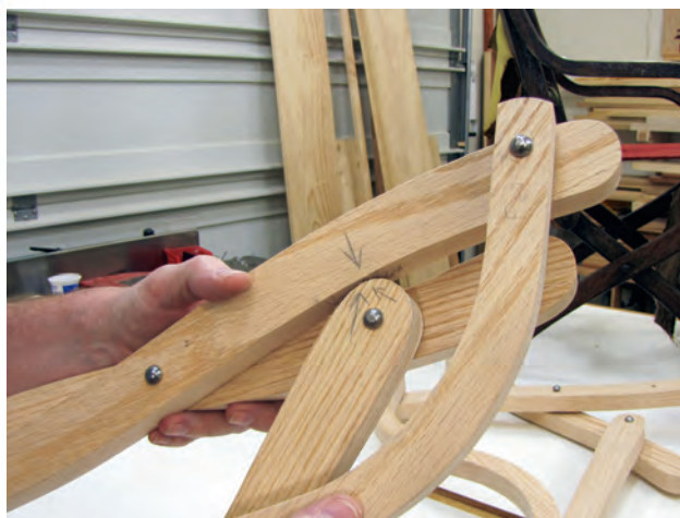
Temporarily insert rivets (photo above) to check the folding action to be sure nothing binds. The author cut the end of one leg just a hair too wide (photo right), causing the lower tip of the backrest to rub at the penciled-in arrows. A little more time on the spindle sander refined the leg to allow for clearance. (Note: rivets were purchased at www.rjleahy.com )
