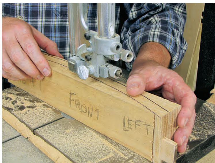
Cut the curves into the stretchers on the band saw. With all the curved parts on this chair, your band saw will get a workout. During the Civil War era, these curves would have been cut with a bow saw by hand.
