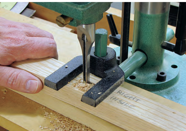
A benchtop mortiser makes short work of cutting mortises into the backrest components. It's easy to cut on the wrong side of mirror-imaged components like these, so it's important to mark everything clearly.
