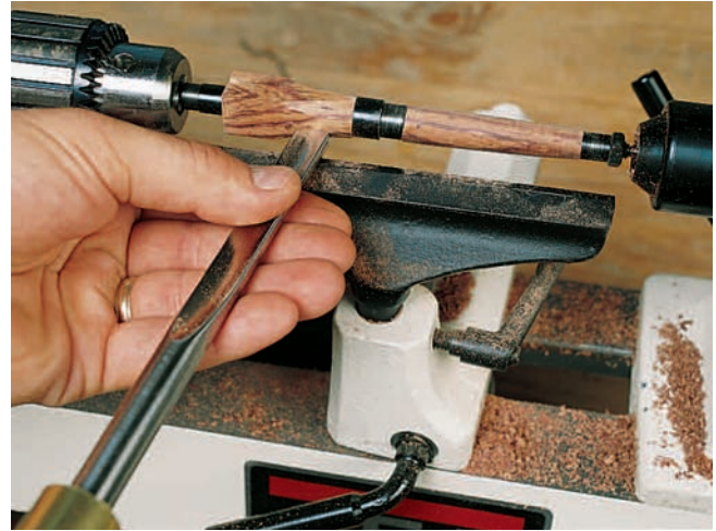
Figure 2: When turning the pen's elliptical shape, don't get aggressive and trim your bushings. It dulls turning tools and makes for very small pens toward the end of a run. Get close and switch to sandpaper.
