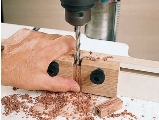
Figure 1: Equip your drill press with a good fence and stop system for this production project. Remember to continually back out the waste as you drill through the blank to prevent splitting.
