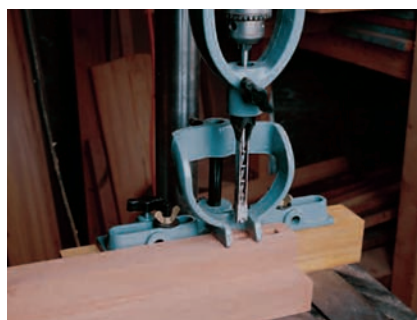
Figure 1: A mortising attachment equipped with a 1/4" hollow-point chisel will form all the mortises for the carcass and doors.
