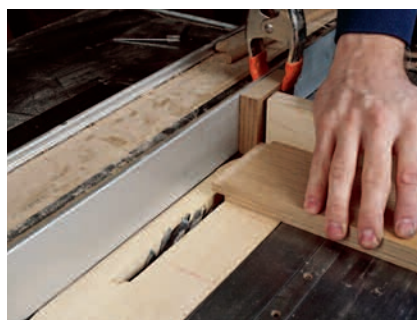
Figure 2: It's easy to cut tenons with a table saw using a miter gauge to support the stock and a set-up block to establish the length of the tenon.
