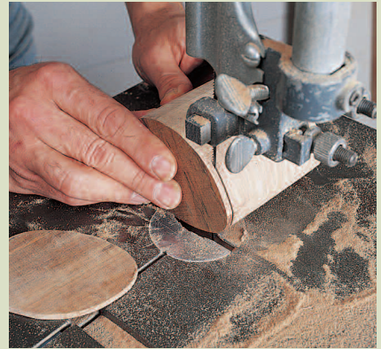
Figure 2: Reset the saw for the depth of the next cut. Carefully slice 1/4"-thick pieces off of each side of the center box section. Hold these cuts as straight and true as possible as these pieces will become the sides of the sliding box.
