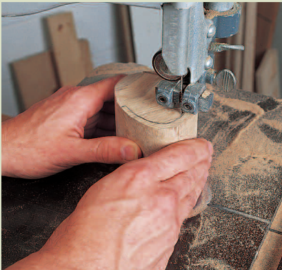
Figure 3: Put the side pieces away for now and again reset the saw to the next depth of cut. Draw lines to guide your cut as you remove the waste from the box. Make the opening as large as possible to allow for the greatest access to the box after you glue the sides back on .
