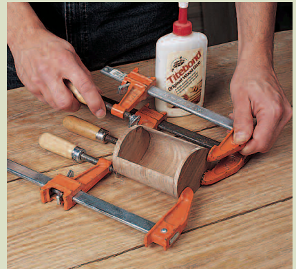
Figure 4: Glue the sides back onto the center section. Sand the project smooth and use a marker or 1/8" dowel of contrasting color to make the eyes. Apply an oil or clear finish. Flock the inside of the box section for a finishing touch.
