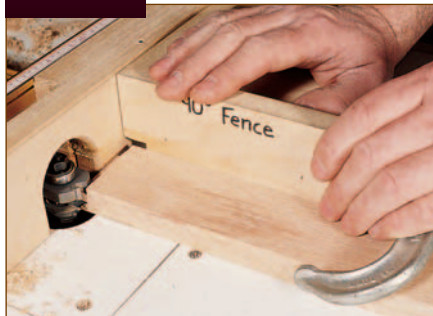
Figure 2: The rail ends are machined to fit into the grooves formed by the first cutter. Then use a raised panel bit (below) to shape both sides of the panels.
