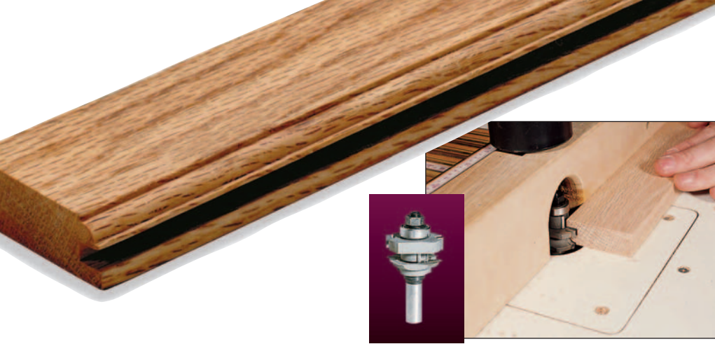
Figure 1: Stile and rail bits are the best way to create the mating joints characteristic of frame and panel construction. With your first pass you'll form a bead and groove.
