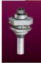
Figure 1: Stile and rail bits are the best way to create the mating joints characteristic of frame and panel construction. With your first pass you'll form a bead and groove.
