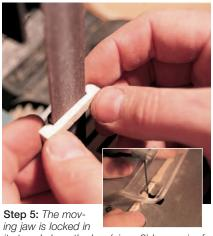
its travel along the bar (piece 3) by a pair of maple wedges (pieces 4). Scroll saw these wedges to rough shape, (see pattern at left) and use a small belt sander or a file to refine the cut. Be sure you don't over-sand the wedges or they'll lose their locking action. This has to be a tight fit.
