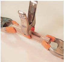
Step 3: Glue the two halves of each jaw together before cutting them to shape. Spring clamps supply enough pressure to snug the halves without excessive squeeze out. To keep glue out of the mortise, insert a piece of scrap exactly the size of your bar into the opening and slide it out before the glue dries.
