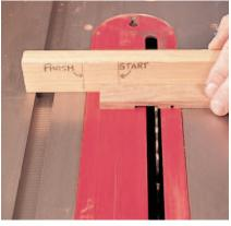
Step 2: Draw a starting line 1%" to the right of the blade on your miter gauge fence and add a finish line 1%" to its right. With the end of a fixed jaw at the starting line, cut out the mortise to a depth of 1/8", as shown above. For the larger mortise in the moving jaw, draw two more lines, each 3/16" further out, to accommodate the wedges.
