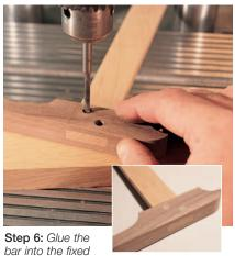
jaw, checking for squareness. Drill the holes for the pins (pieces 5), glue them in place and sand flush when the glue dries. Glue the cork (pieces 6) to the jaw faces and apply your finish. Slip the movable jaw and wedges onto the bar and tap a stop (piece 7) in place near the end of the bar.
