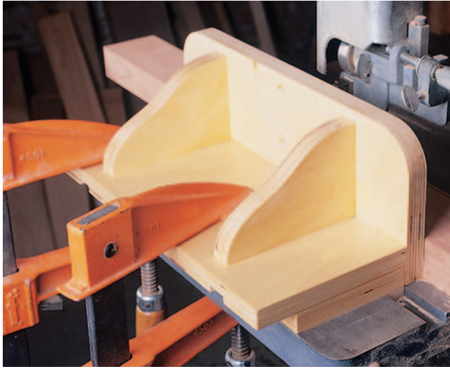
Figure 1: For ripping operations or resawing stock that's been milled four-square, the fence alone may be all the guidance you need.
