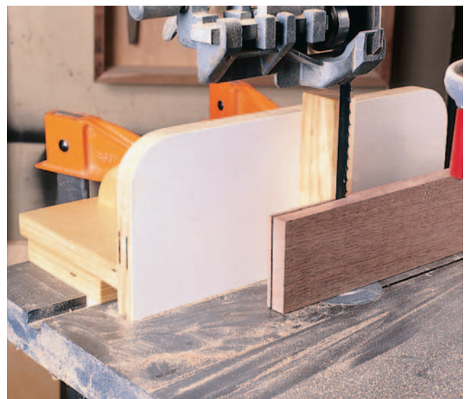
Figure 2: When working with a dull blade that tends to drift or when cutting along a scribed line, add the single point attachment so you can pivot your stock slightly for easier tracking.
