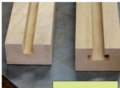
After plowing a simple groove into the slide member, expand the slot with a T-slotting router bit.
