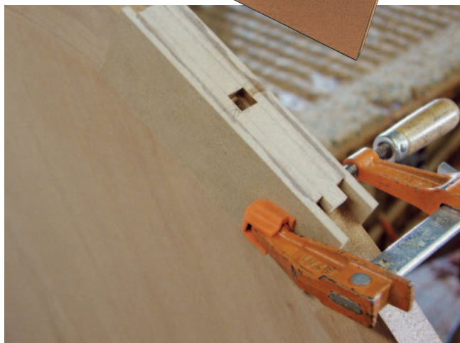
Routing the mortises into the rim for all the ebony plugs is achieved using a small clamped-on jig. The router is outfitted with a 1/4" bit and a 3/8" o.d. rub collar.
