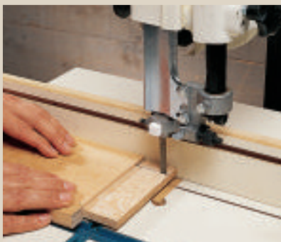
Cut the tenons to thickness and length with a dado blade on the table saw, then make the end cheek and shoulder cuts on the band saw. Guide your work against a fence.
