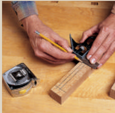
Lay out all the leg mortises with a combination square before you begin milling them. This will help keep their order and orientation clear on each leg.
