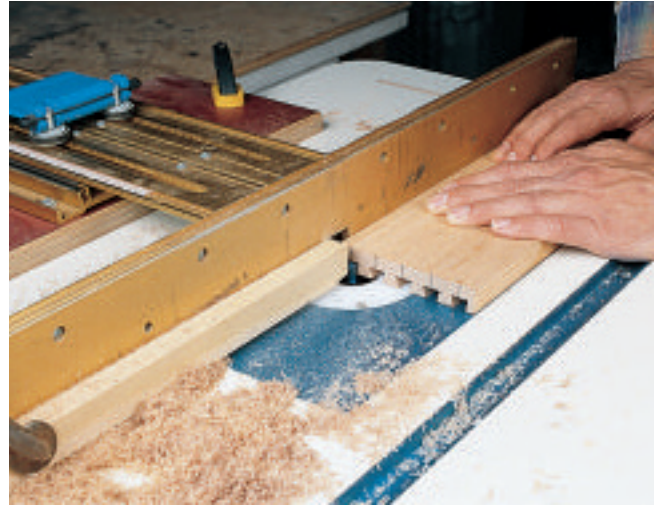
Mill tails into the drawer face to complete these half-blind joints. On this jig, a stopblock clamped to the fence limits the depth of the cuts.
