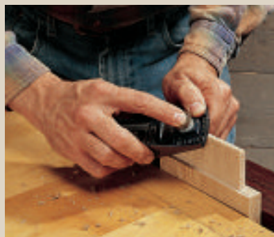
Take shavings off the tenon until it fits its mortise, then chamfer the ends and edges. The chamfers help smooth the assembly and become distinctive visual details.
