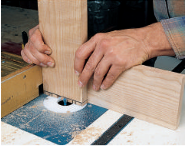
Rout evenly spaced pins across the sides with a dovetailing jig and 1/2" dovetail bit. Test the setup on scrap before cutting the actual parts.
