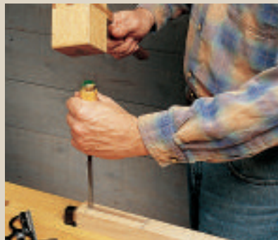
Square up the mortise ends with a chisel and mallet. For deep through mortises, a mortising chisel works best. Keep the chisel held square to the leg as you tap it home.
