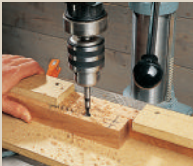
Clamp the hold-down jig to the drill press table so the drill bit spur is centered inside the mortise. Drill a series of adjacent holes along the mortise to remove the waste.
