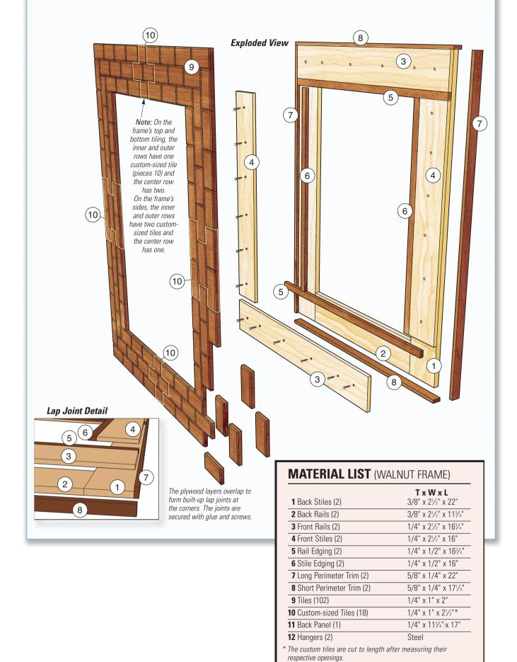
Tile chamfers are formed with a 1/8" roundover bit (Rockler #28429).
