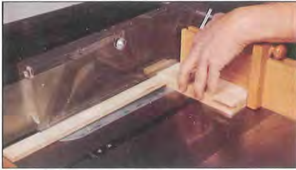
Photo D: Trim the jaws to uniform length on the tablesaw.
