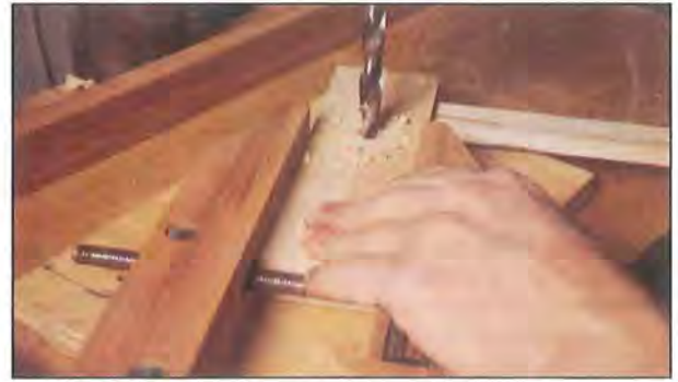
Photo E: Bore 1/2" holes to radius the notch ends.
