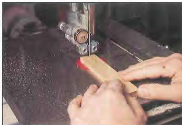
Photo B: Bandsaw the cam notch on the end of the jaw center.
