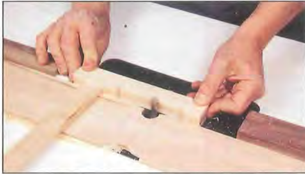
Photo F: Rout the notch edges using stops to limit travel.
