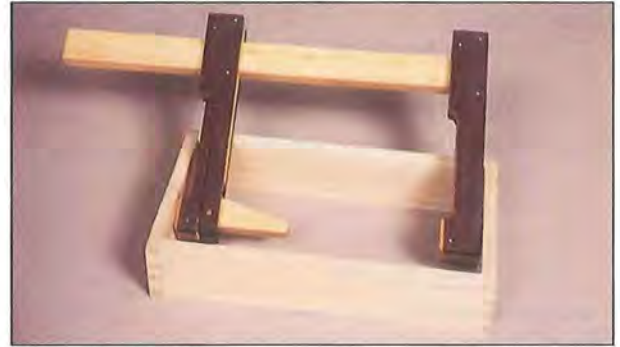
Photo G: Reverse the movable jaw to use clamp as a spreader.
