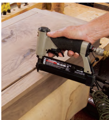
Pin the door onto the hinged portion of the box with a pin nailer (above). Then flip it open and drill pilot holes through the door backer into the door. Attach the door with screws (right), covering the heads with self-stick felt dots, which cushion the door when it closes.
