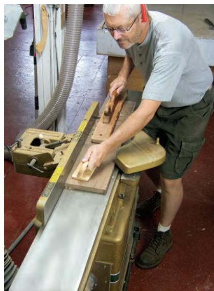
Joint and plane your stock square and flat before gluing up the book-matched panel. Surface the panel to final thickness last.
