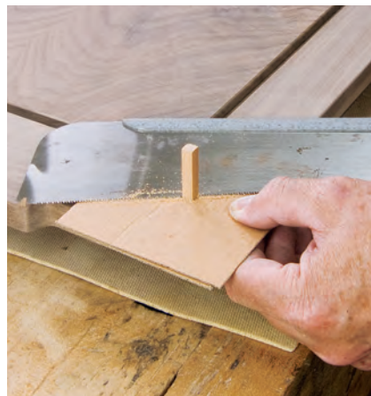
Bore shallow door peg holes before chopping them square with a hollow-chisel mortising bit. Line up the chisel with squared-off marks surrounding the hole. Use a wooden mallet to protect the chisel. Tap lengths of cherry pegs home. Try using cardboard with a hole in the middle to gauge the peg length and to protect the door frame during the final trimming and sanding stages.
