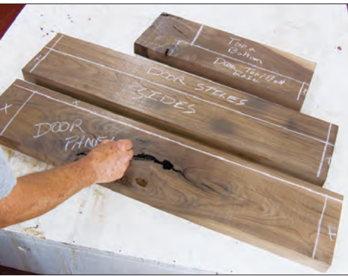
Plan your cuts with chalk, reserving the best figure for the door panel (top). Scribe a centerline down the edge of the board with a marking gauge to use as a guide for resawing (right). Close, double lines are even better.
