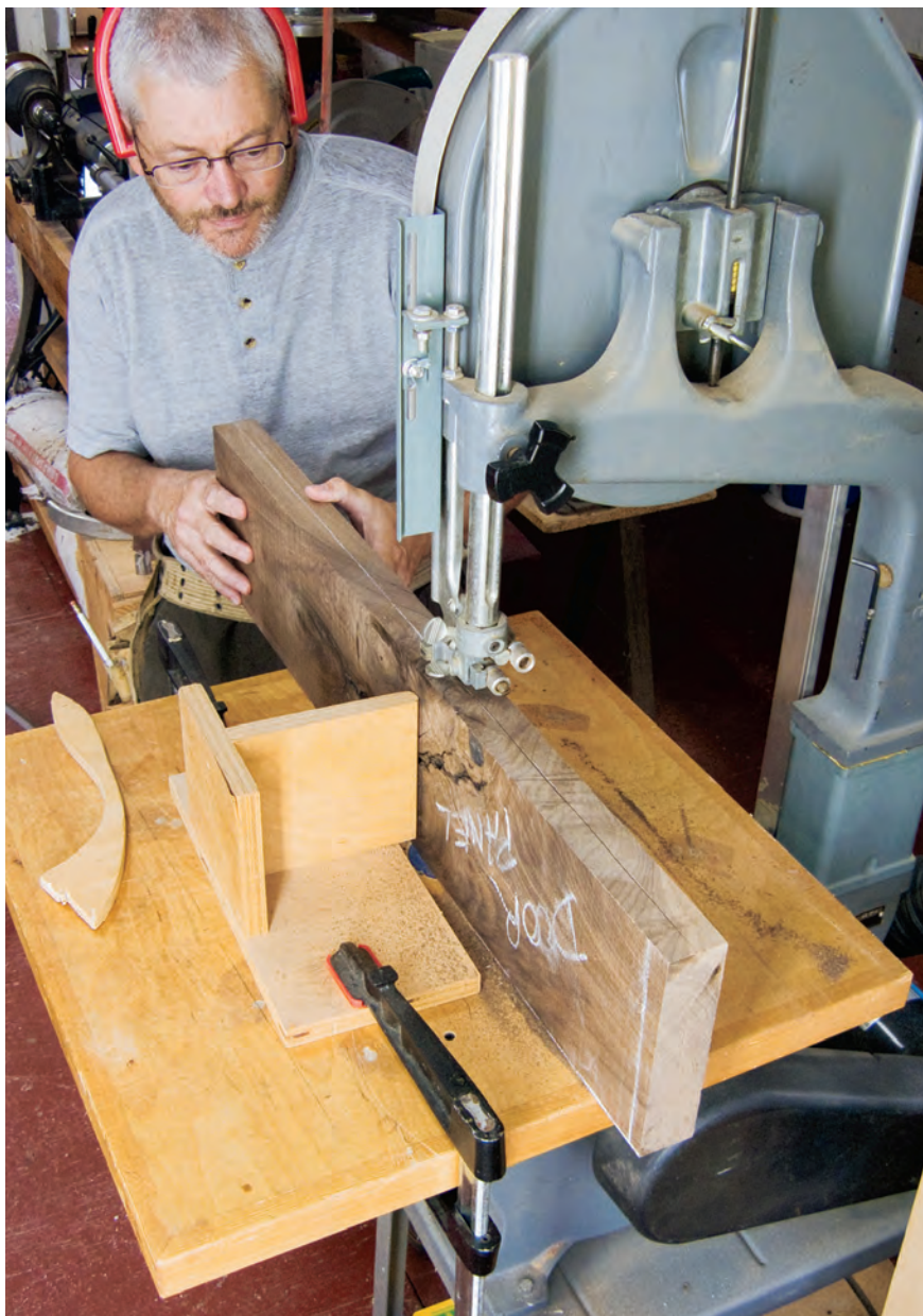
Resaw thick stock with a single-point fence. The beauty of this fence is that it allows you to swing the wood to account for blade drift and still keep your blade tracking right down the middle. Have a push stick within easy reach to safely finish your cut.
