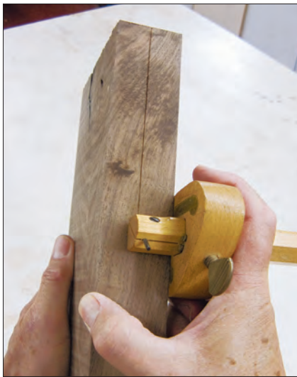
Plan your cuts with chalk, reserving the best figure for the door panel (top). Scribe a centerline down the edge of the board with a marking gauge to use as a guide for resawing (right). Close, double lines are even better.
