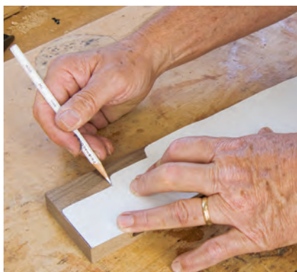
Transfer the top door rail profile onto the rail with a paper template. A white colored pencil is easier to see on dark wood (left). After band-sawing this piece to shape, you'll find that a small rat-tail file is just the ticket for shaping the slight inside curves, as shown at right.
