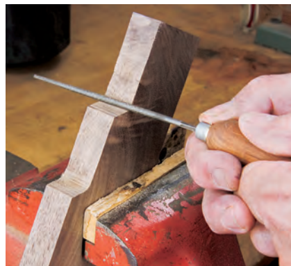
Transfer the top door rail profile onto the rail with a paper template. A white colored pencil is easier to see on dark wood (left). After band-sawing this piece to shape, you'll find that a small rat-tail file is just the ticket for shaping the slight inside curves, as shown at right.
