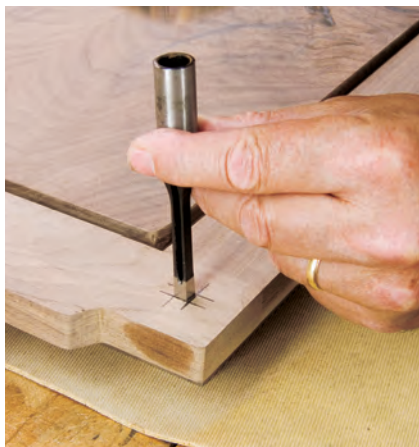
Bore shallow door peg holes before chopping them square with a hollow-chisel mortising bit. Line up the chisel with squared-off marks surrounding the hole. Use a wooden mallet to protect the chisel. Tap lengths of cherry pegs home. Try using cardboard with a hole in the middle to gauge the peg length and to protect the door frame during the final trimming and sanding stages.
