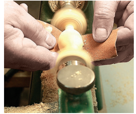
To make painting easier, sand the plugs all the way up to 400-grit sandpaper.
