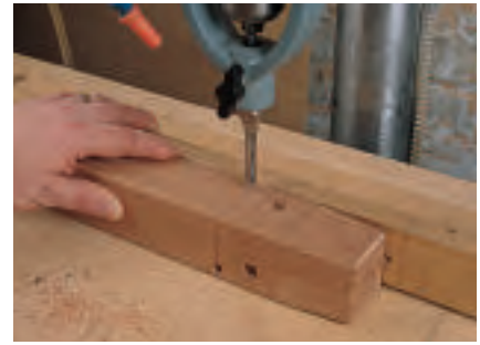
Install a mortising attachment on your drill press to create the square mortise for the legs' decorative ebony plugs.
