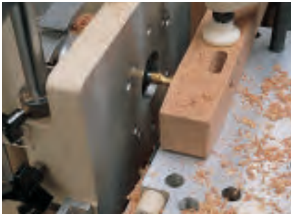
Mike chops his mortises with a Multi-router. This project's mortises are all conventional straight mortises that can be formed just as easily in the traditional manner.
