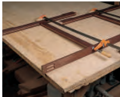
Begin assembling the pedestal's side sub-assemblies as shown above. Note the top rails' orientation and pocket screw joints.
