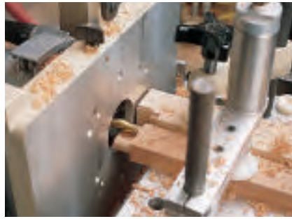
Tenons on the panel dividers are shorter than those on the bottom rails. Test-fit the tenons in their mortises as you make them.
