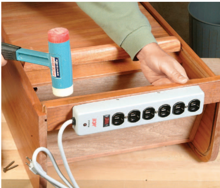
One of the last steps is to drive home the cabinet's bottom rail. A power strip is mounted to the rail. It provides electricity to all the battery chargers.
