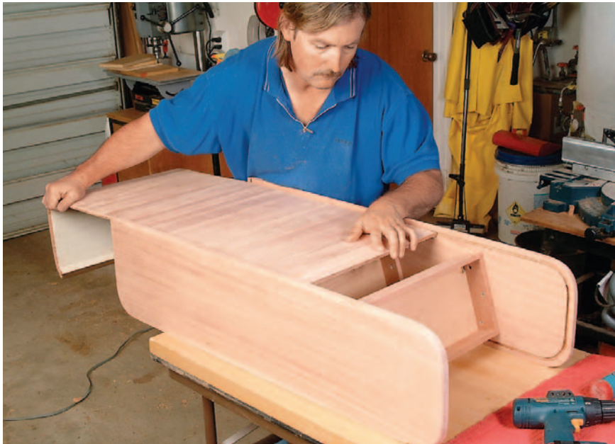
With the cabinet assembled, gently slide the tambour door into its track. This step will require a bit of patience and care, since even slight racking or one misaligned slat can hang things up. If the door sticks, slide it back a nudge and try again.
