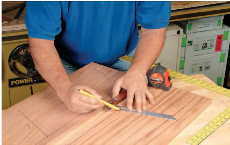
Use a sharp carpenter's pencil and a bevel gauge set to 70° to mark out where the tray bottoms meet the cabinet sides.
