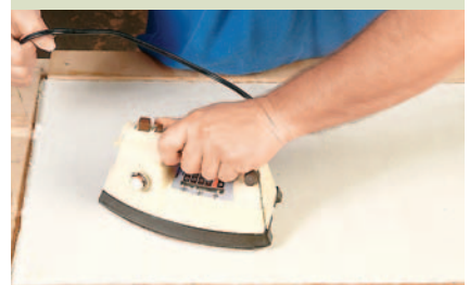
Quick-set the glue with a hot iron. After the glue has cured,
