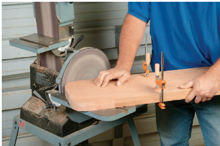
Use a disc sander to smooth the corners of the sides to the marked radii. The goal is to end up with three 1/4-round, identical corners on each cabinet side.
