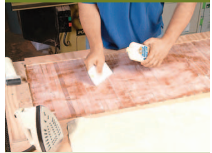
Quickly apply a thin layer of glue (yellow or white woodworking glues work equally well) to one side of the canvas and then the slats. (This takes quite a bit of glue.)
