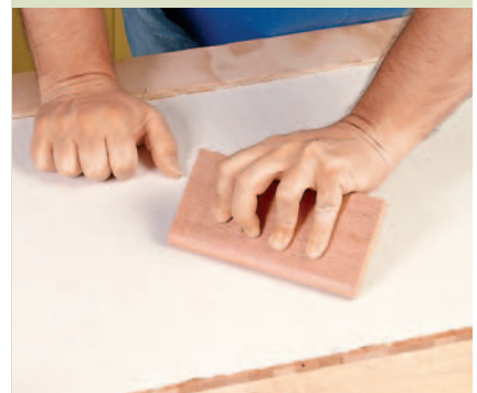
Place the canvas on the slats, aligning the trimmed long edge to the long stop of the jig (don't worry if the glue starts to dry; ironing will reactivate it). Press the canvas flat using a round-edged block of wood.
