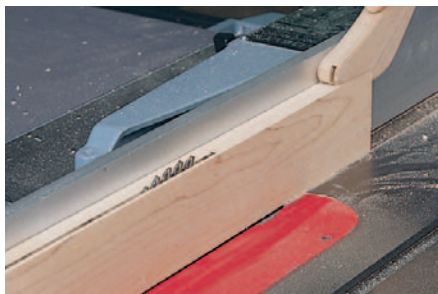
Figure 4: To resaw \frac{3}{4} " stock, use a pushstick and make a number of \frac{1}{2} "-deep passes until the blade pokes through the top edge of the stock.
