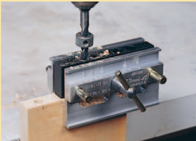
Figure 2: Lay out the dowel locations on the cabinet sides, then position your doweling jig. Slipping a stop collar onto the drill bit will limit the depth of the holes.
