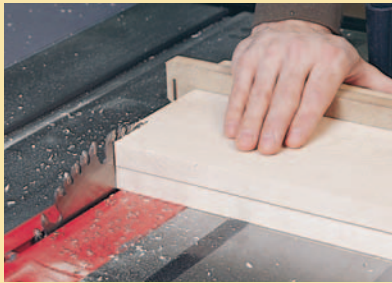
Figure 1: Stack any pieces that need to match and crosscut them to length at the same time. This will ensure a square cabinet assembly.
