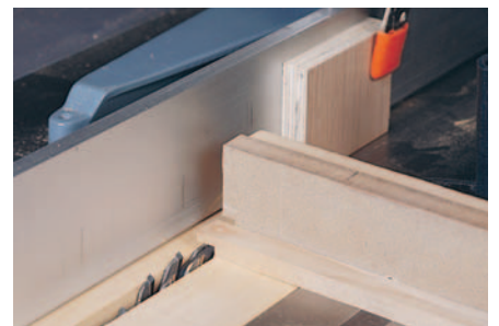
Figure 5: After cutting the mullions to length for your door, cut exactly half way through your stock with a \frac{5}{16} " dado blade to form the tenons.
