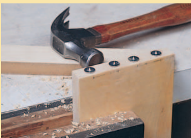
Figure 3: To transfer the dowel hole locations, insert steel dowel centers in the sides and press them into position on the top and bottom pieces.
