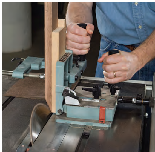
Using a band saw (top photo), trim away most of the 22½° mitered joint waste. Then make the finished cuts using a table saw and tenoning jig. Rough cutting the joints first eliminates the risk of creating nasty flying projectiles.
